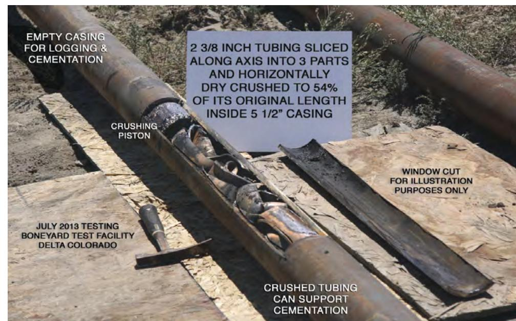
Similar to the picture on the left, Oilfield Innovations' method slices tubing into spaghetti-like strands that can then be severed with a conventional cutter and crushed with a conventional inflatable packer acting as piston, which is placed through the tubing and inflated between the severed and shredded ends.
