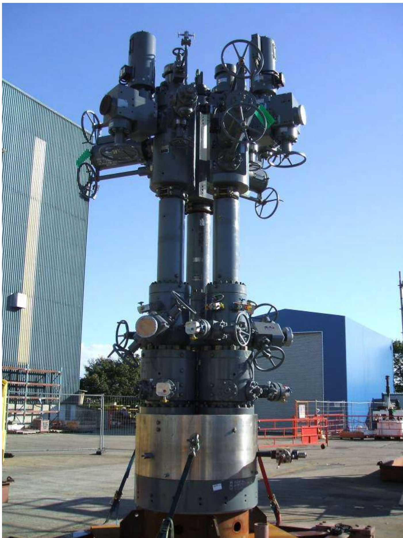
Figure 12 - Britannia Triple Wellhead Arrangement (Matheson, 2008) 11
