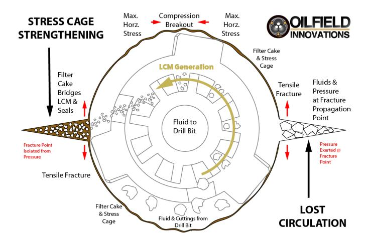
Figure 1 - Lost Circulation and LCM Generation Explanation
