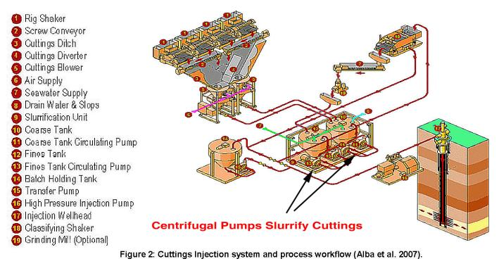
Figure 2 - Proven Technology of Cutting Slurrification<sup>2</sup>
