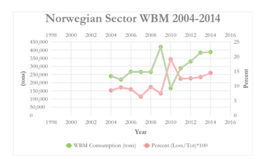
Figure 4 - Water Based Mud Consumption and Loss<sup>3</sup>
