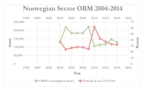
Figure 5-Oil Based Mud Consumption and Loss <sup>4</sup>
