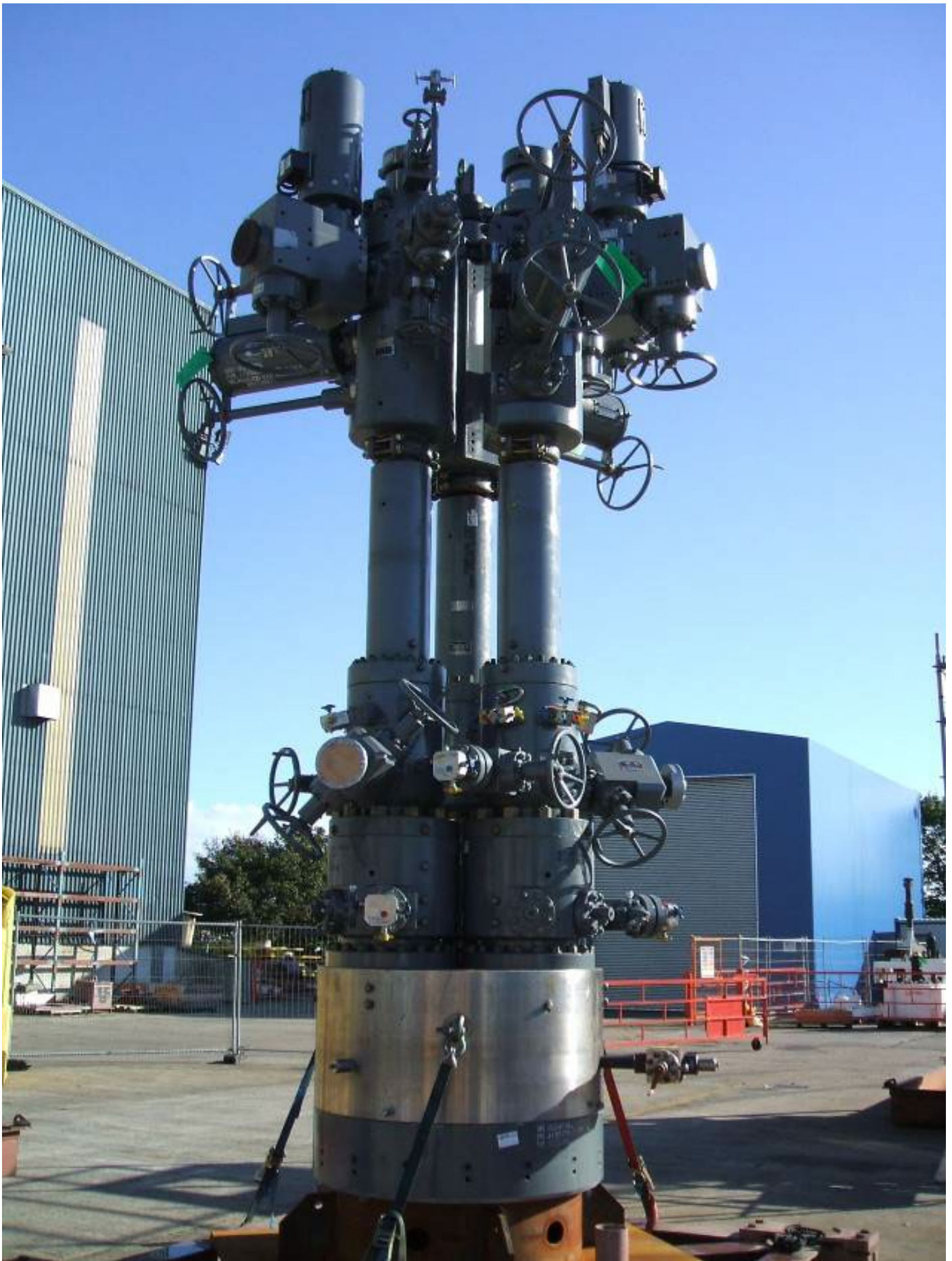
Figure 17 - Britannia Triple Wellhead Arrangement (Matheson, 2008) 11
