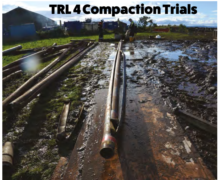
9.625 Csg Piston Area = 57.2 in 2 4.5” API 12.6-ppf L80 Tubing
