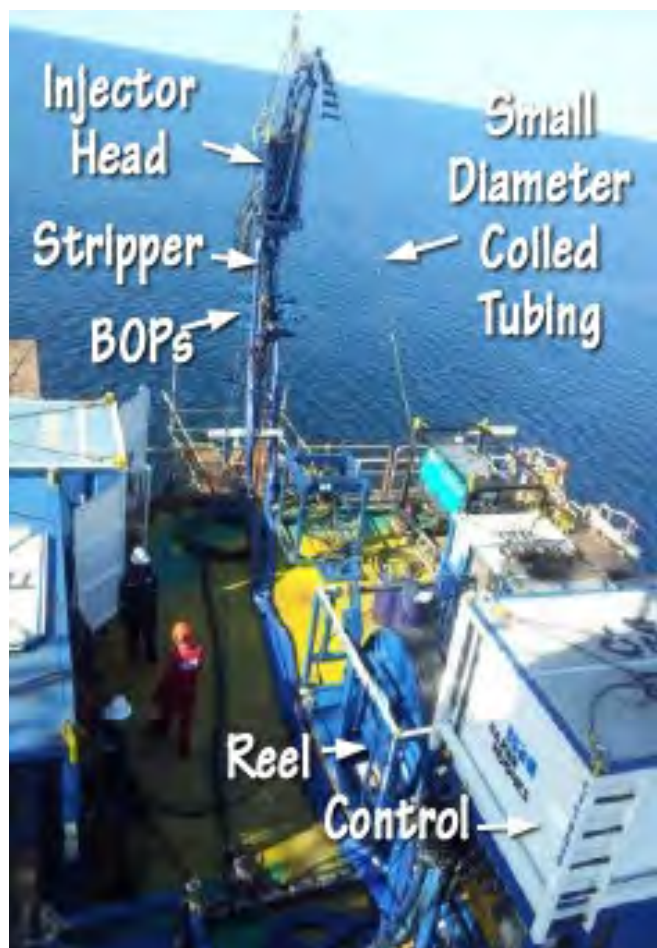
Figure 30 - Rigless Coiled Tubing on Limited Space Small Platform (Sundramurthy, 2014) 45
