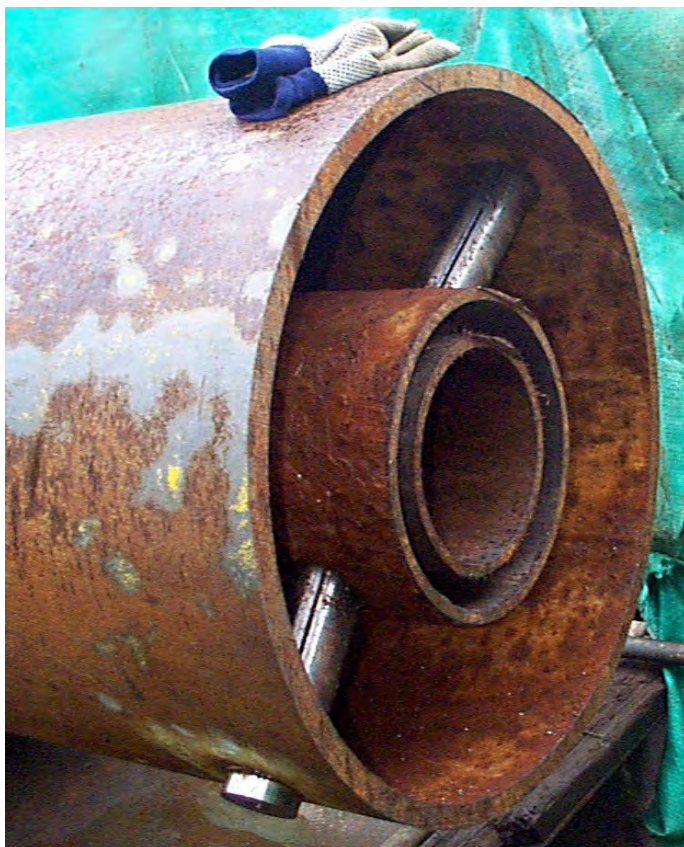
Figure 35- Pinned Well Conductor and Casing (Phillips UK Ltd,2001) 96
