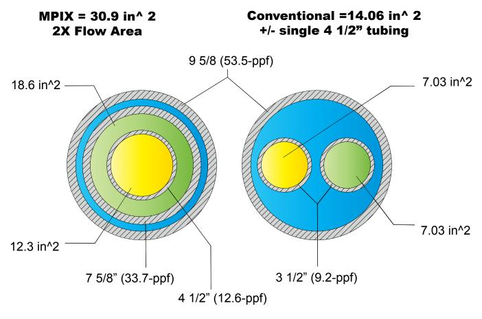
Figure 1 - Comparison of MPIX to Conveniontal Dual String Completions
