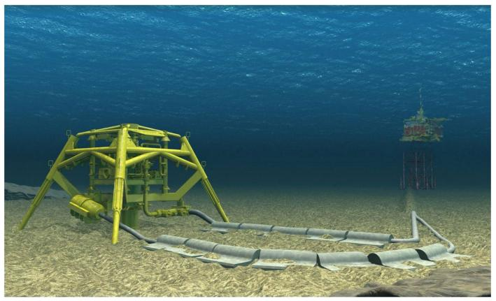
Figure 13- Subsea Tie-Back
