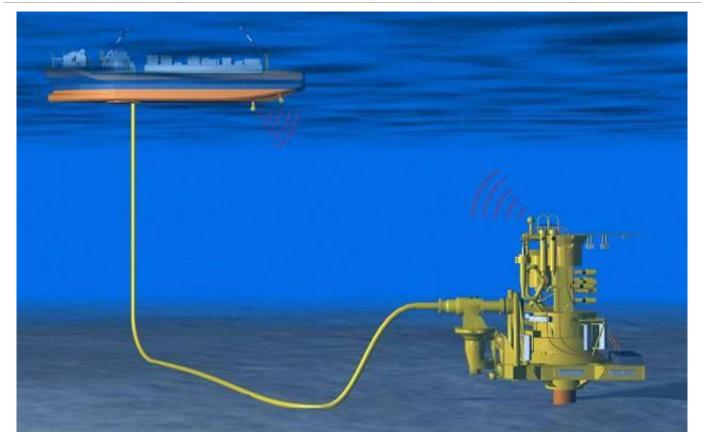
Figure 11- Single Subsea Well Tie-Back
