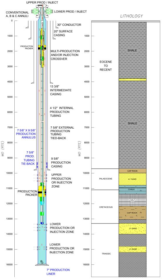
Figure 10- MPIX Single Bore Completion in Vertically Stacked Reservoir
