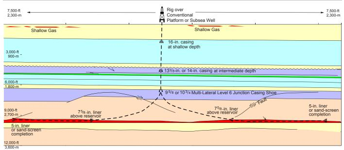
Figure 8- Multi-lateral extending to Laterally Separated Reservoirs
