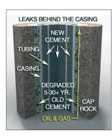
Historically, drilling rigs and pulling units have removed tubing from subterranean wells so that oil and gas companies could log and confirm the integrity of the cement behind the casing they placed through the cap rock before finally cementing the internal portion of the casing.
