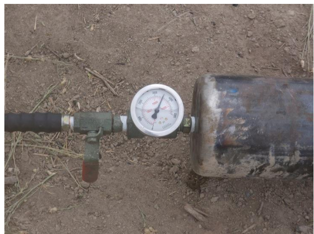
Figure 3 – Pressurized Wet Piston End
