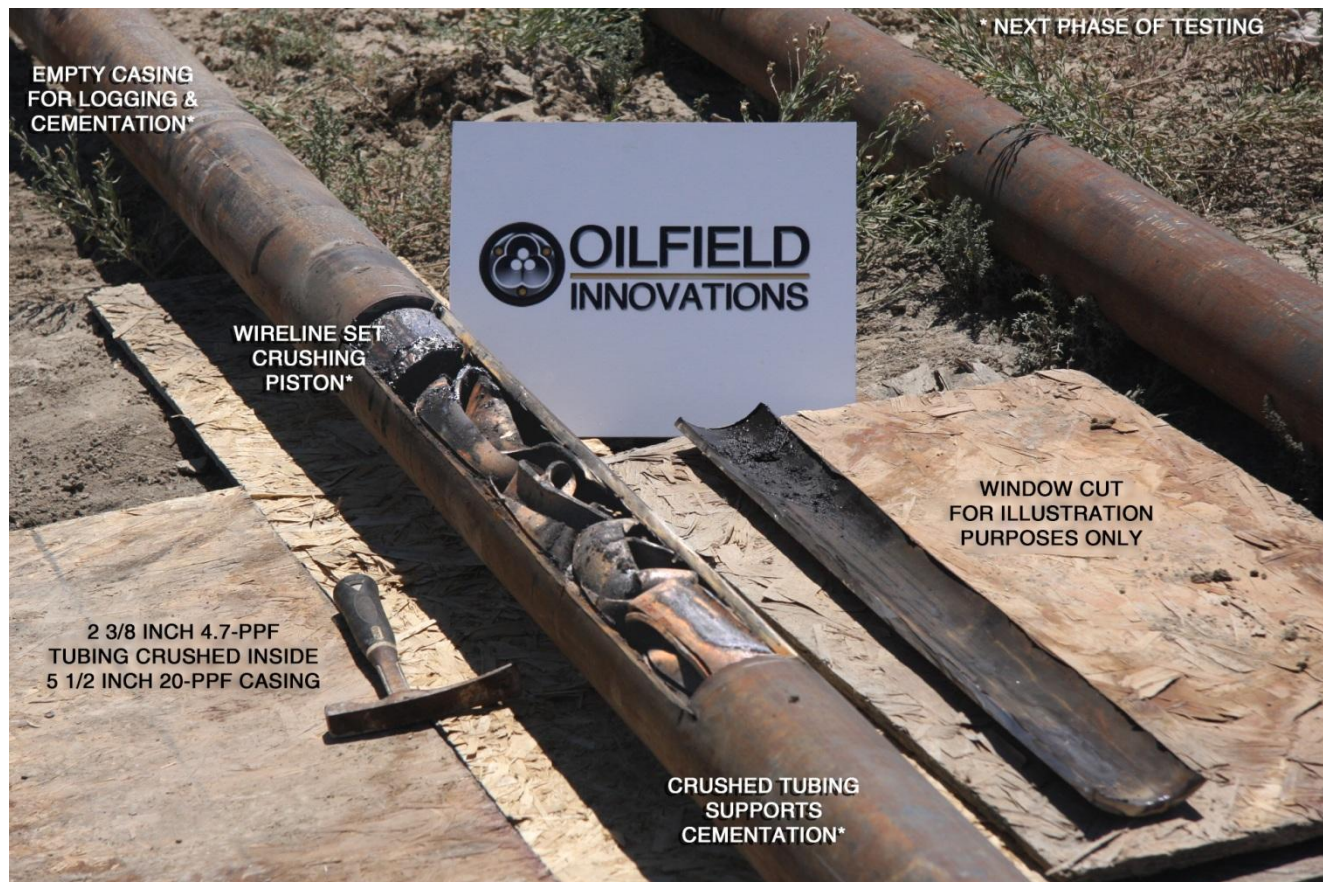
5 Figure 1 – Modelling Run [5] Crushed 2 3/8” Tubing viewed through a window cut in 5 1/2” casing.
