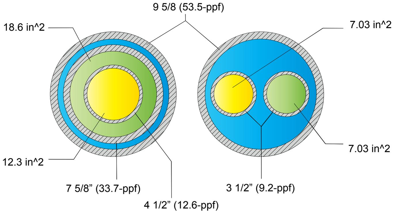
*Figure 1 - Comparison of MPIX to Conventional Dual String Completions*
