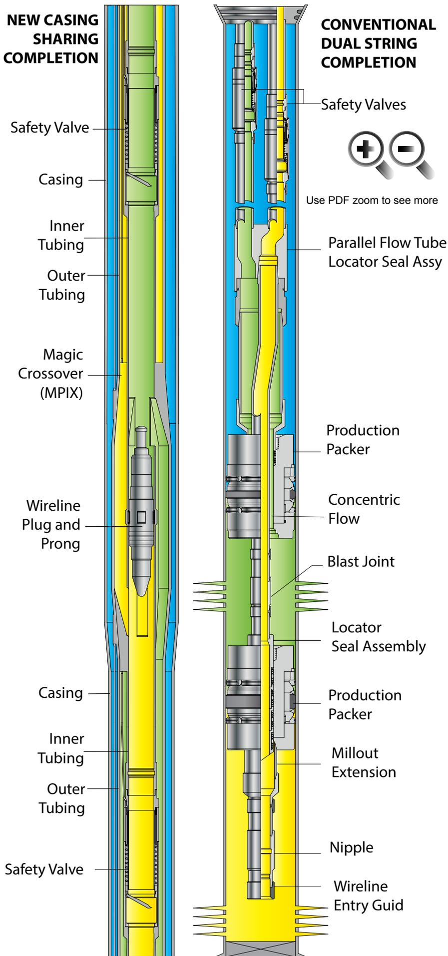
Figure 2 - Comparison of MPIX to Dual String Completion
