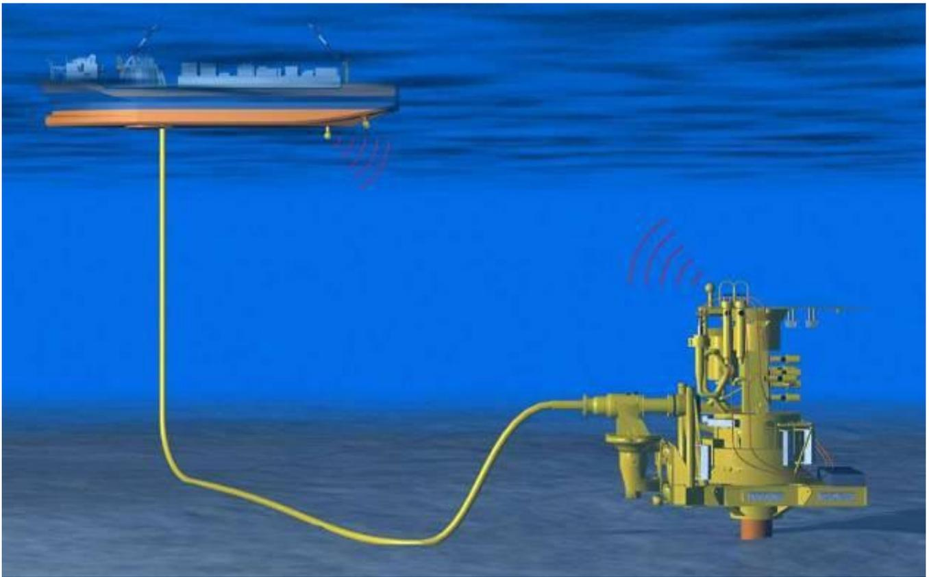
*Figure 11- Single Subsea Well Tie-Back*
