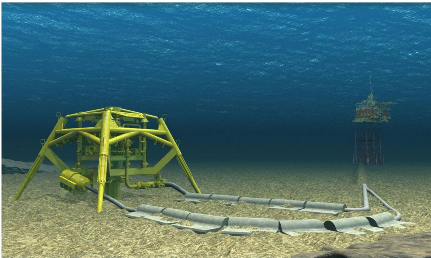
*Figure 13- Subsea Tie-Back*
